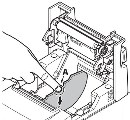
**Note:** After using a paper roll with a width of 57.5 mm, do not change to a paper roll with a width of 79.5 mm. (This is because the printer head has deteriorated as a result of a portion of the head having been in direct contact with the platen.)
